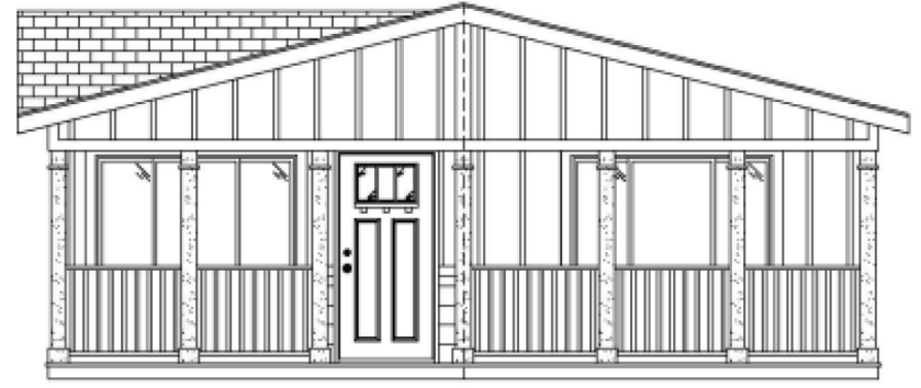
Front Elevation 5/12 Roof Pitch
